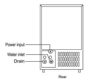
Water inlet and drain has a 3/8" connection
