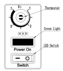
The numbers on the temperature control 1-7 reflect the relative temperature setting from high to low.
